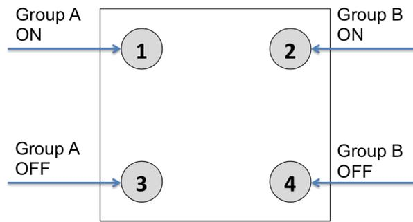
**4 Groups are controlled with two buttons and double click (parameter 1 or 2 => 2)** This mode enhances the previous mode and allows to control two further control groups C and D using double clicks.
