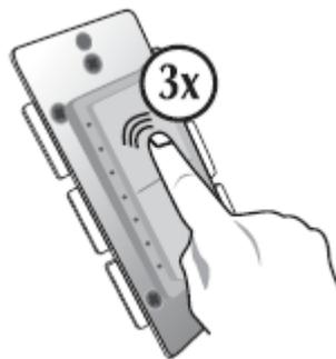
Then, quickly tap the bottom side (OFF) of the rocker 3 times
