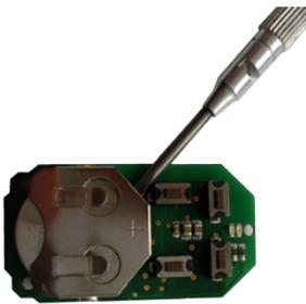
For battery change the device needs to be opened by removing the three little screws on the backside of the device. Use a screwdriver or any other usable device to gently push out the
