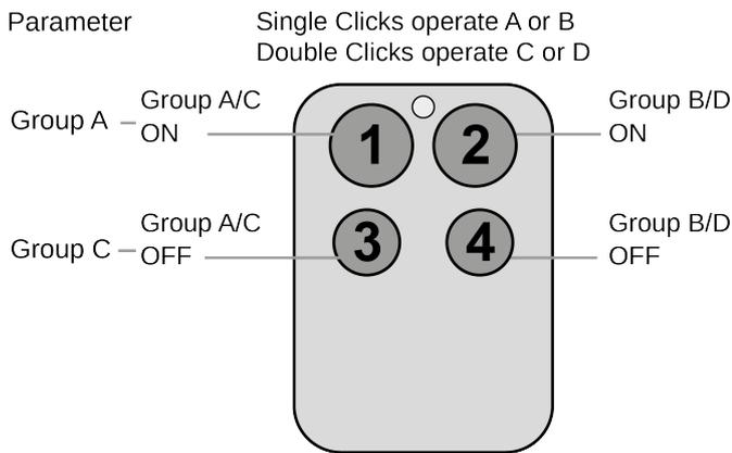
The devices supports 8 different operating modes - this means the kind of command sent out when pushing a button. Operating modes either directly control other devices or they issue various scene activation commands to a central controller. Operating modes for direct device control are:
