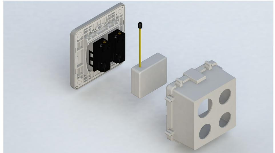
1. Put the in wall PAN08 into a wall box and connect the AC power wire L,N to PAN08 connector L, N.
