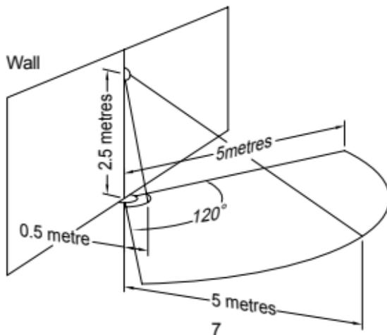
For optimal performance, your MultiSensor should NOT be mounted directly on or near metal framing or other large metallic objects. Large metal objects may weaken the Z-Wave wireless signal MultiSensor depends on for communication.
