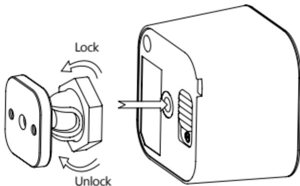
3. The Back-Mount Arm may be locked at various angles by turning the Friction Lock clockwise and counter-clockwise to respectively tighten or loosen the angle of the arm. You can rotate the Friction Lock to change the measurement area of sensor.
