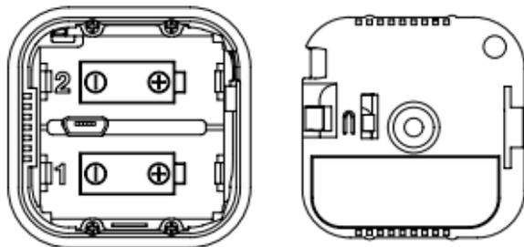
2. Insert the smaller end of the provided USB cable into your sensor's USB port.
