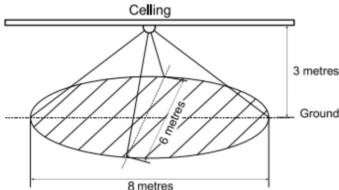
If installing MultiSensor in a corner where the wall meets the ceiling it can take measurements within a 2.5 x 5 x 5 metres / 8 x 15 x 15 feet range:
