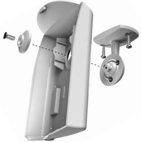
FIG 3. Installation of the optional Deluxe Swivel Bracket.
