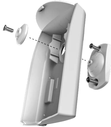
FIG 2. Installation of the Standard Swivel Bracket.
