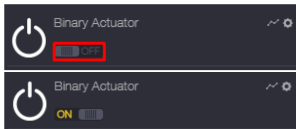
Image 62 Switch being turned on
