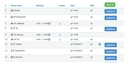
In case the device interview and configuration was not performed properly a little question mark icon will indicate this. Clicking on the question mark will open a window displaying the details of the interview process. The correct loading of a Device Description File is indicated as well. For battery-operated device the time of the last wakeup, the time of the next wakeup and the current wakeup status is shown. Clicking on the table heads reorders the table view of the data.
