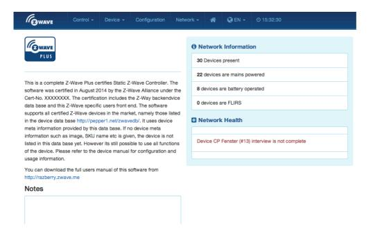
The Network Information box offers some statistics about the number of devices in the network and how many of them are mains or battery operated. The network health box will list devices that have problems: the battery is down, the interview is not complete or the device failed. Clicking on the statement will lead to a help page explaining the problems and giving guidance for remediation.
