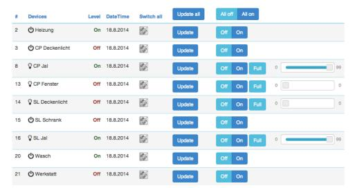
All actuators can be switched on or off. Dimmer and motors controls can be operated using a slider. For dimmer there is a button "On" and "Full". "Full" turns the dimmer always to 100 % diming value while "On" will turn to the last dimming state before the dimmer was turned off. Clicking on the table heads reorders the table view of the data.
