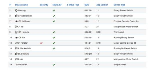
The type info dialog lists all devices of the network and indicates if they support enhanced Z-Wave functions such as Security and Z-Wave Plus. Their Z-Wave protocol version, their application version and their device type indicator is shown for information purposes too. Clicking on the table heads reorders the table view of the data.
