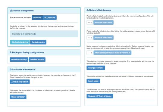
Please refer to the devices manual on how to do an inclusion. In case the inclusion does not work as expected, please exclude the device first. More than 90 % of all inclusion problems are caused by still included in a different network and can then not being included again.
