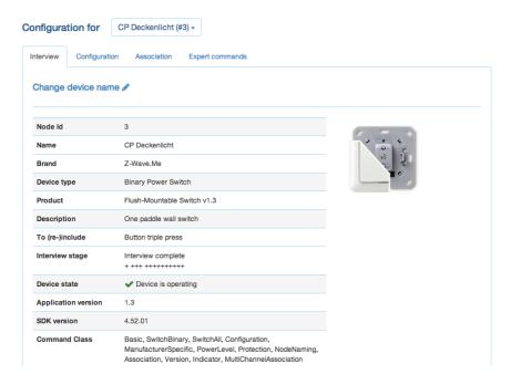
The device interview section shows the result of the device interview. In this process the controller tries to get information about the device. In case the controller find a device description record for the device it will display further information about the device that can not be obtained from the device itself. If the software will not automatically recognize the device and load the description record a button "Choose Device Description Record" allows to do this manually.
