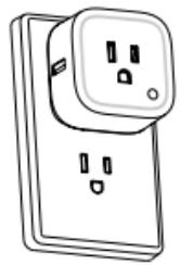
When the Smart Switch is plugged into a wall socket and powered on, it can act a repeater in your Z-wave network
