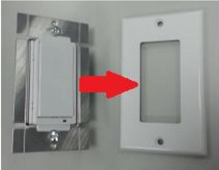
Step 3, place the bottom case of ZSC to the In-wall switch. **Make sure the existing switch is in ON position.**
