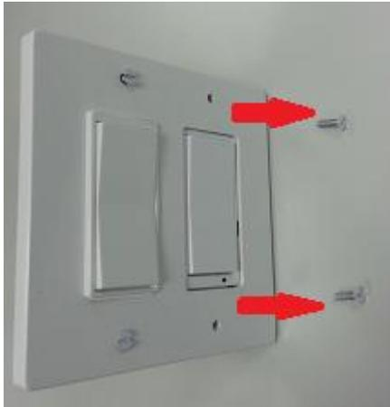
Step 2, place the bottom case of ZSC main unit on top of the existing faceplate. **Make sure the existing switch is in ON position.**
