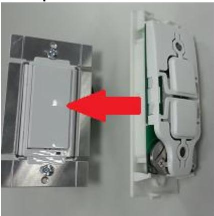
Step 4, tighten the mounting screws and secure the bottom case of ZSC
