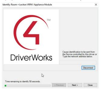
3 Identify (add) the Z-Wave device according to the manufacturer's instructions, usually by pressing a Z-Wave button on the device. See the documentation for the Z-Wave device for more information.
