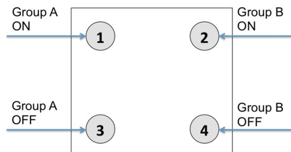
**4 Groups are controlled with two buttons and double click (parameter1 or 2 => 2)** This mode enhances the previous mode and allows to control two further control groups C and D using double clicks.
