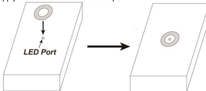
2. The sensor head has built-in magnet. Apply the sensor head to the washer to attach the sensor to LED port for reading LED pulse from watt hour meter
