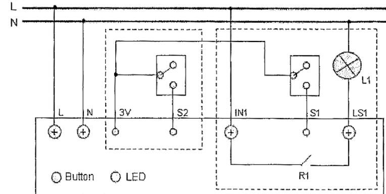
As illustrated in the above diagram, S1 provides a wall switch connection to the dry contacts. By default S1 switch supports Single-Pole-Double-Throw (SPDT) type of binary switch. However, through the setting of Gateway, S1 can be configured to support Toggle switches as well. The S2 switch can also switch the on/off status of the unit when toggled.
