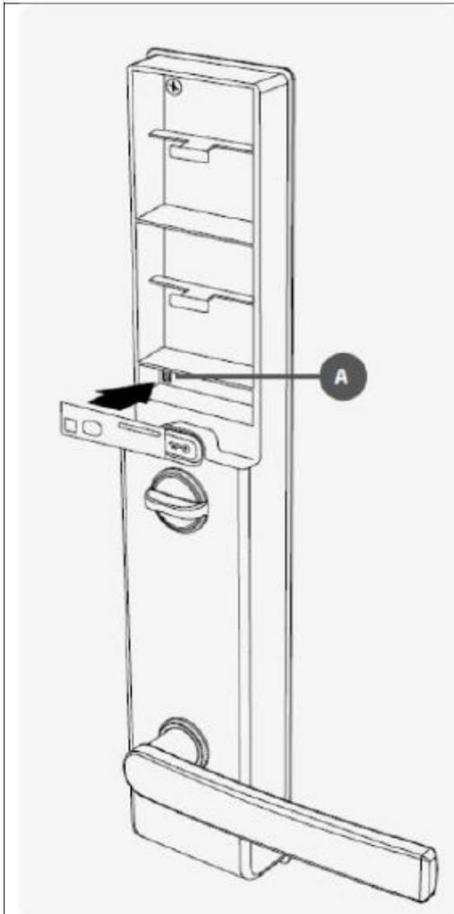
**IMPORTANT:** Batteries must be removed prior to removing or inserting the interface module.
