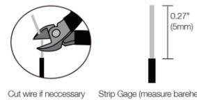
Note: All connection wires needs to be flexible cable.
