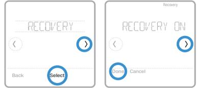
When Adaptive Intelligent Recovery is active, you'll see the recovery symbol in the upper-right corner of the thermostat screen.
