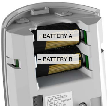
Correct polarity shown
