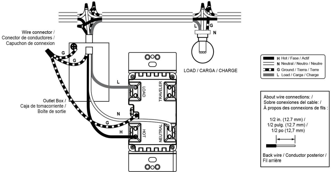
**Figure 2: SQR14102\*\*Z 3-Way Wiring Diagram with Mechanical Switch**
