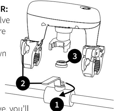
**3. INSERT THE SPACER IF NEEDED:** when installing the Titan on a low-profile valve, you'll need to place the included spacer accessory between the valve handle and the Titan's fork.
