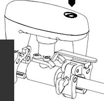
The unique SmartStart QR code is printed on the back of the product and on the side of the packaging (don't use the QR codes from the manual for SmartStart). The LED indicator will flash quickly and beep to signal communication. It will turn solid green for 3 seconds if inclusion is successful.
