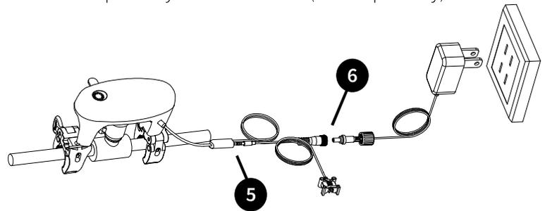
**6. POWER THE ACTUATOR:** connect the power jack on the included DC adapter with the Titan's power cord. Turn clockwise until the seal cover is fully secured. Plug into a standard 120 V receptacle. The LED will start blinking green.
