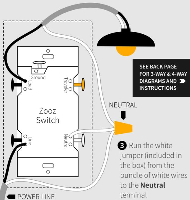
**DON'T FORCE THE SCREWS.** Look up to see how to install the wires correctly.
