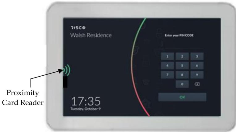
Figure 7: RisControl Screen with Proximity Tag Reader
