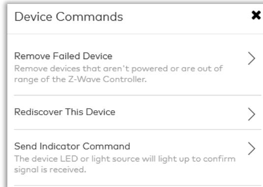
If the Z-Wave device receives an Indicator Set command with the Indicator ID 0x50 (identify), it will identify itself. The identification method will differ based on the hardware available. Identification methods are listed below.
