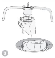
Rotate the handle 180° to the other side of the lock.
