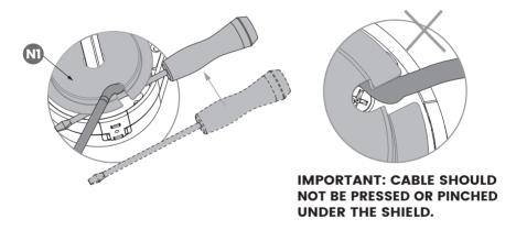
Pull the cable towards the direction of the arrow.
