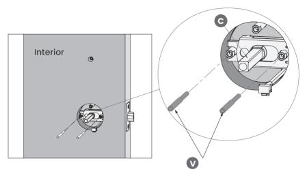
Install Fire Shield as shown. Ensure that the cables are routed out of the U-shaped slot and the fire hood does not press cables.
