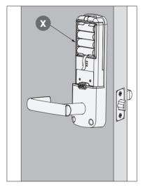
Secure the battery by sliding the Battery Cover **Q** over the lock and turning the screw clockwise on top until tight.
