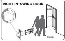
Install Latchbolt **F** to door and secure with Screws **G**. Make sure the spindle shaft is at the center and horizontally positioned.
