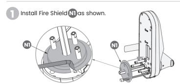
Insert a screwdriver under the fire shield to support while carefully routing cable to the U-shaped notch.
