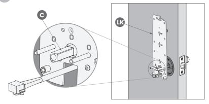
Secure Interior Mounting plate with Screws O, Remove the Position Rods Oand replace them with Screws Tighten clockwise until the
