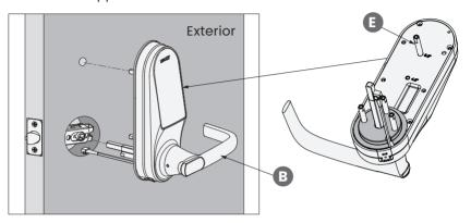
Pass the Spindle C through the center of the latchbolt, and the round rods through the sides in their respective holes. The cable should run underneath the lockset.
