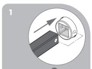
Install Spindle © with the holes side into the base of the lock and align the holes locate in the 3 o'clock and 9 o'clock position.
