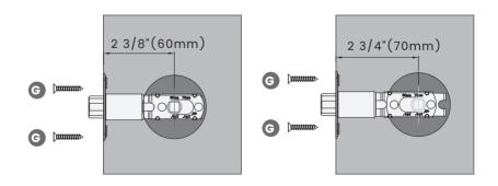
The lock ships with handle default for right in-swing or left out-swing door. Check the diagram below if you are unsure of you door orientation.
