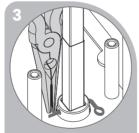
Carefully bend the end of the locking pin **D** with a needle nose pliers.
