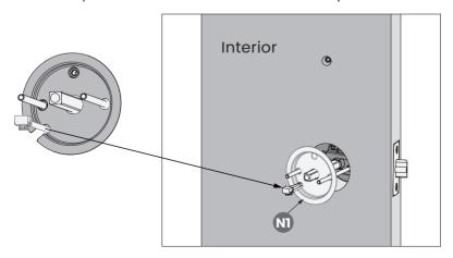
Cable and Spindle © passed Mounting Plate (k).
