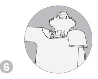
Twist key back to horizontal position. The key can be taken out once it goes back to the horizontal position.
