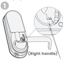
Insert key and rotate so that the two white dots align as shown.
