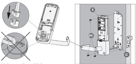
Make sure the cable is away and not tangling with the Spindle C
