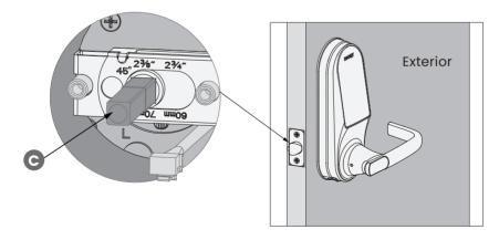
Check lock alignment and ensure that it is sitting flat and aligned straight.
