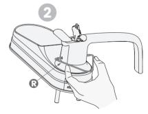
Use the provided pin insert  $\mathbb{R}$  to press the metal pins located at the 3 o'clock and 9 o'clock positions on the base handle. Remove the handle once the pins are compressed.
