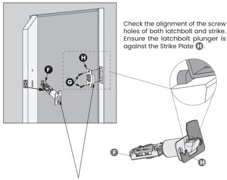
Make sure the slanted side of Latchbolt **(F)** is closing against the slanted part of Strike Plate **(H)** before fixing it on to door frame.
