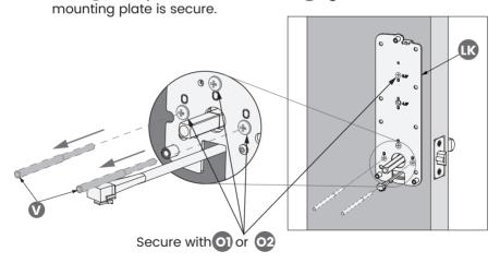
O1 KM4 x 25mm, for door thickness, 1 3/8"~ 1 2/3" (35~43mm)
