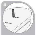
Insert Slotted Barrel Extension (E) to upper hole of the exterior assembly. Use pliers to securely tighten (E) clockwise.
